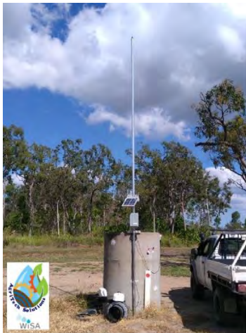
WISA field radio used to control field valves (Source: Agritech Solutions)
