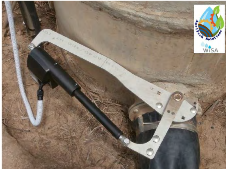
Linear actuator controlled by radio to open and close valves (Source: Agritech Solutions)
